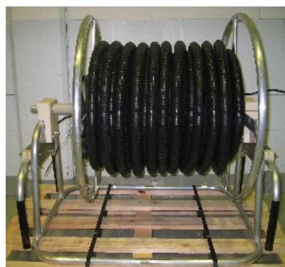
Floating cable on reel
